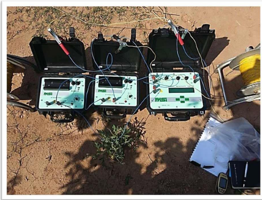
Figure 49. Field data acquisition Resistivity Meter by PASI (Italian Company) By using the apparent resistivity data of ERSS curves, Earth Resistivity Models of 17 resistivity probes and geoelectric parameters including Transverse resistance (T) and Longitudinal conductance (S) are evaluated with several modeling iterations (ERSS-1 through ERSS-17) as given below:
