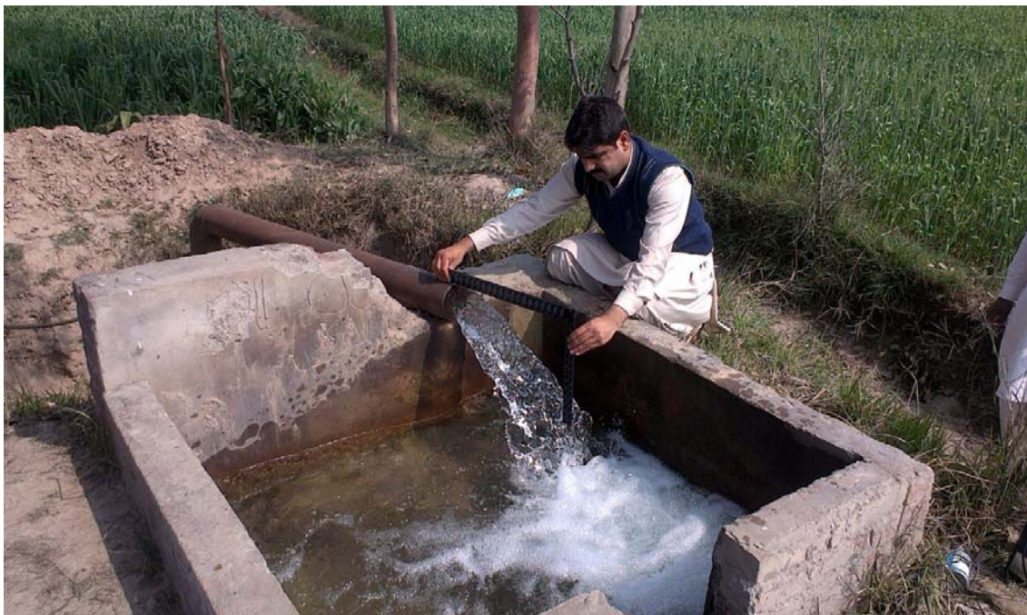
Figure 5.8: Measurement of Discharge by Coordinate method
