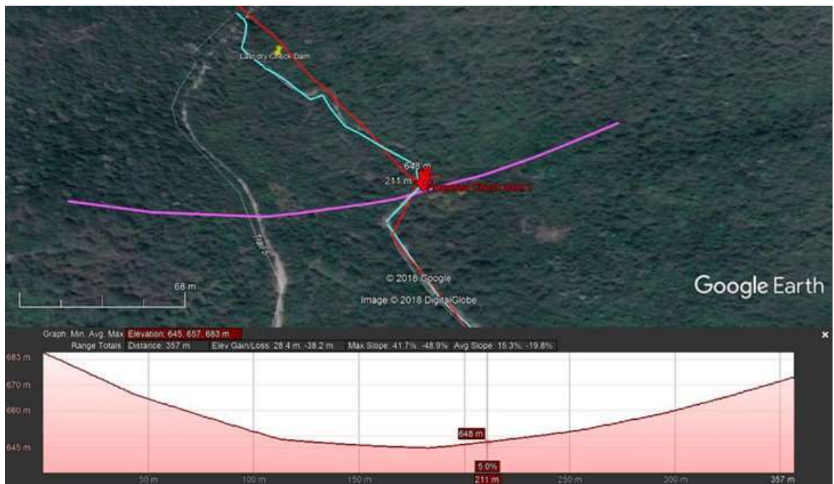
Figure 7.9. Cross section at Proposed Check Dam 1
