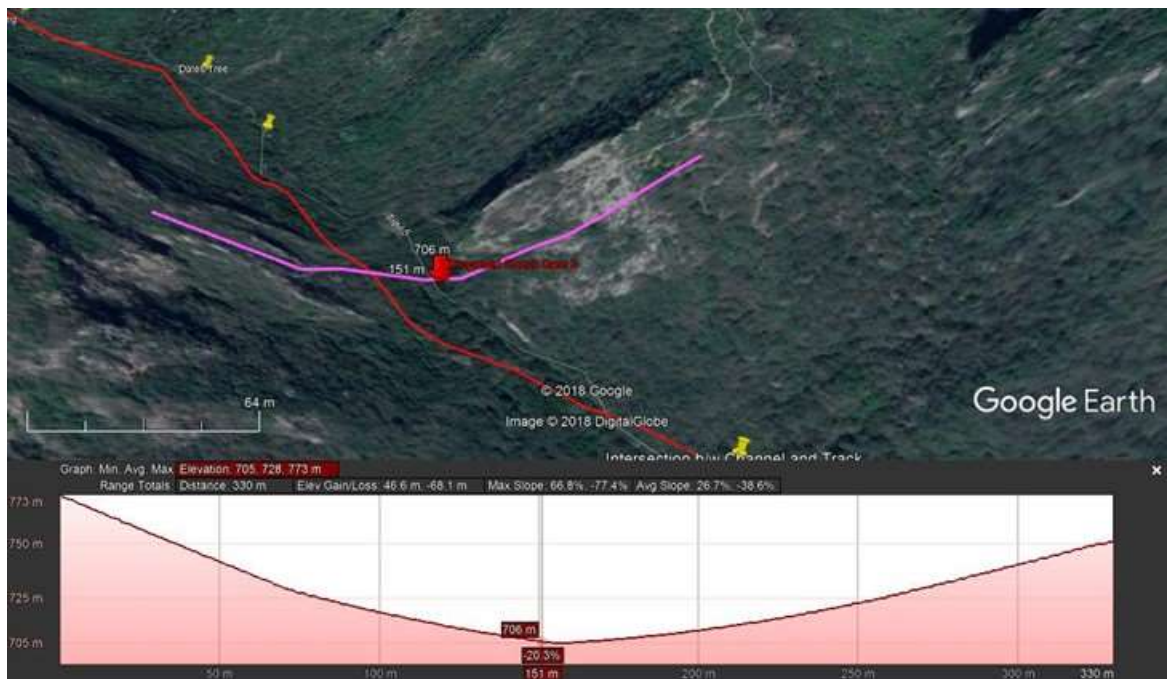
Figure 7.10. Cross section at Proposed Check Dam 2
